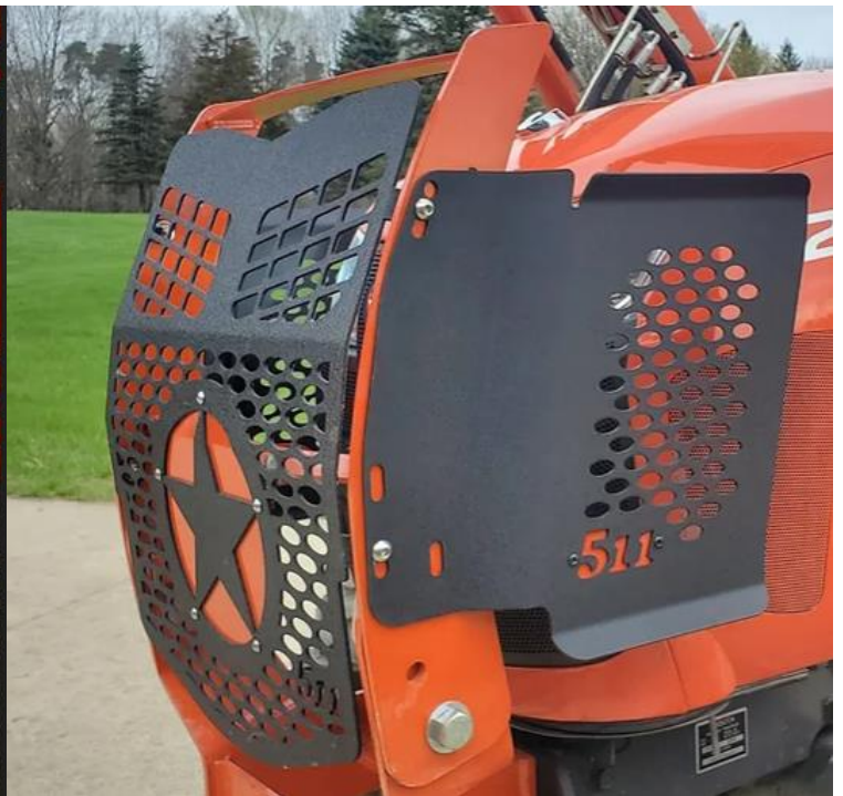
Completed installation with side guards
