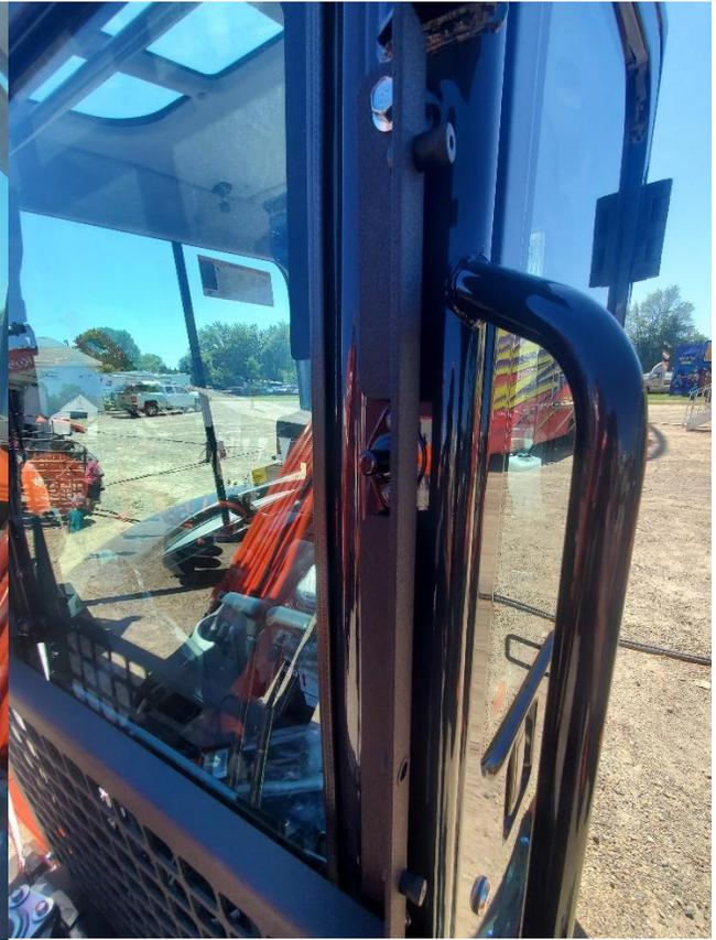
*Figure 2 Left Side Mounting Rail*
