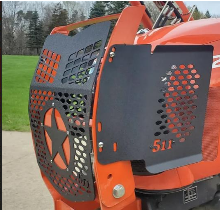
Completed installation with side guards
